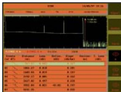
**Bottom Screen** Ideal for long haul supertrunk testing, the DR OTDR module has over 35dB dynamic range. On a very long fiber, MTS allows the user to easily step along the trace from event to event.
